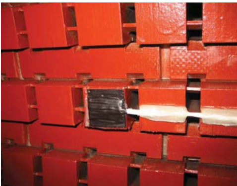
Fig. 4 Flux Probe (black) mounted on a stator core tooth, with connecting lead (white)
