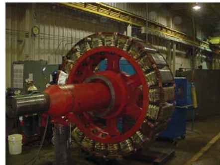
Fig. 1 Rotor from a salient pole synchronous motor
