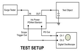
The Iris Power PDAIert Bantam instrument is connected between the surge tester and the test object with as-short-as-possible leads.
