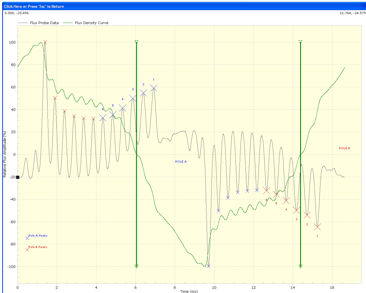
Figure 3. Typical two pole rotor flux measurement
