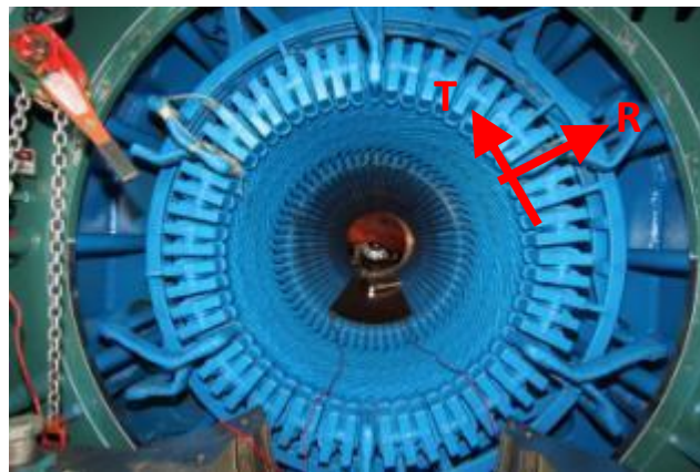
Figure 1. End View of Generator Stator with Radial (R) and Tangential (T) directions
