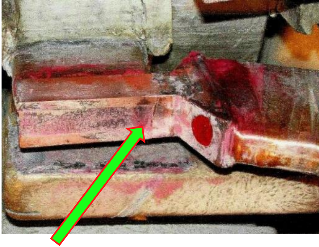
“Phase lead connection crack”
