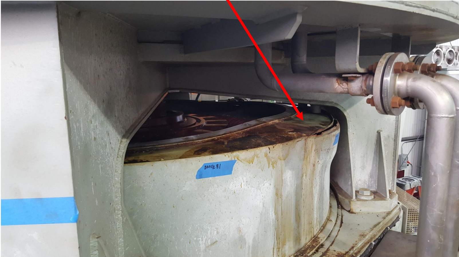
Damaged Endwinding Air Baffle Cover from Ejected Rotor Retaining Ring
