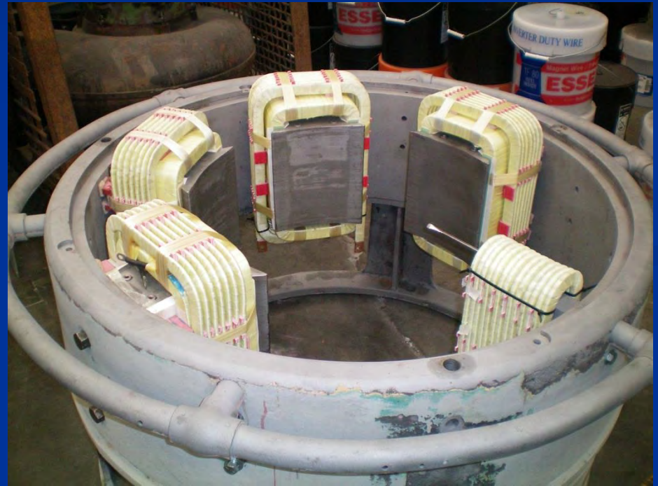
Main Field ,Series Field and Interpole windings
