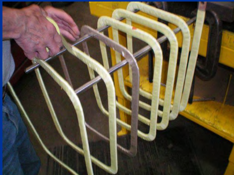
Series Field and Interpole windings ( have a few turns) and Main Field winding ( has many turns).
