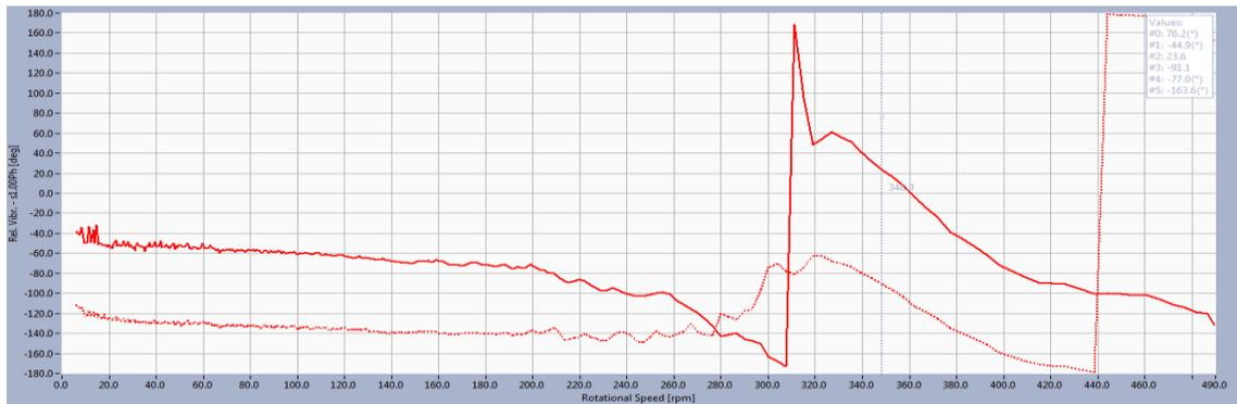
Figure 7 Bode Plots - S1n amplitudes and phases vs RPM;
