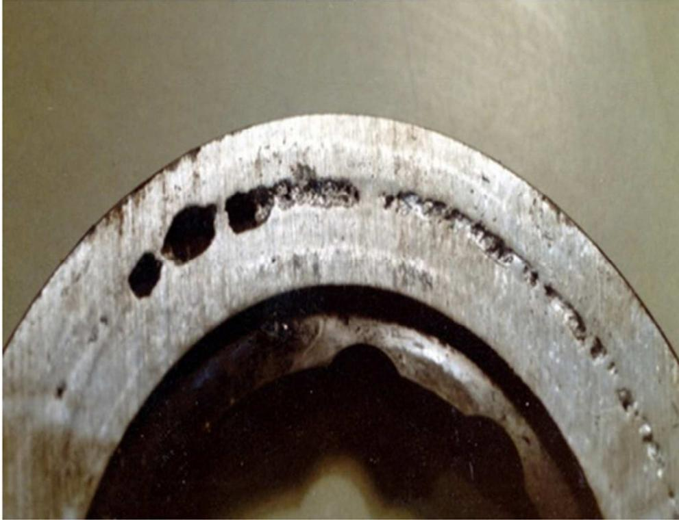
Fig. 3 Die cast rotor with air voids (courtesy of EASA)
