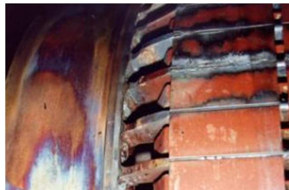
Fig. 2 Rotor core burning from broken bars
