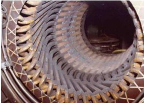
Fig. 4 (b) Stator core damage due to rotor rubbing stator
