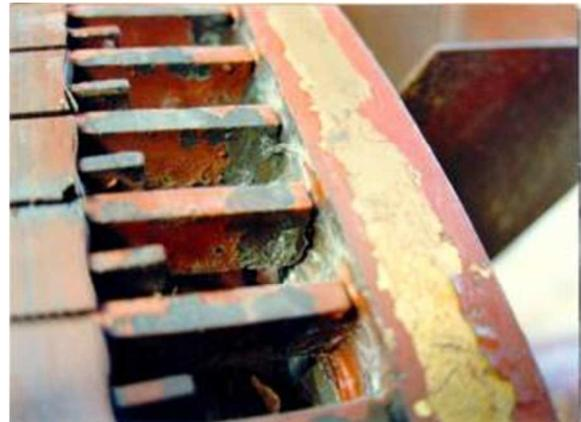
Fig. 1 Failed brazed connection [3]
