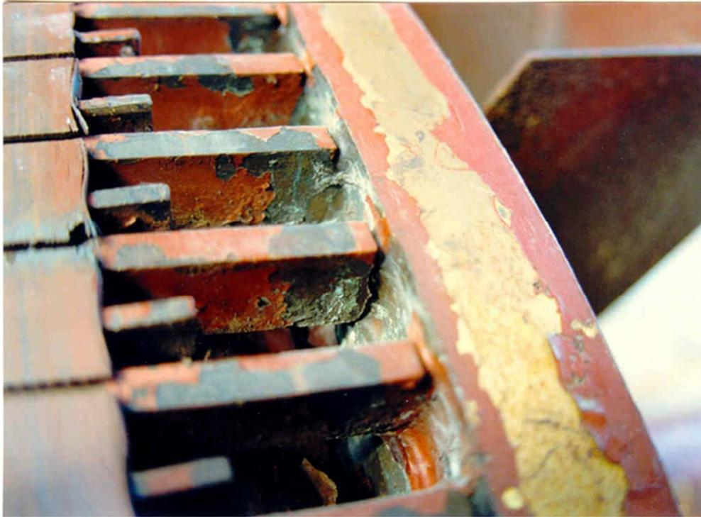
Fig. 1 Failed brazed connection [3]
