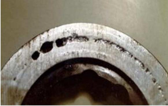
Fig. 3 Die cast rotor with air voids (courtesy of EASA)
