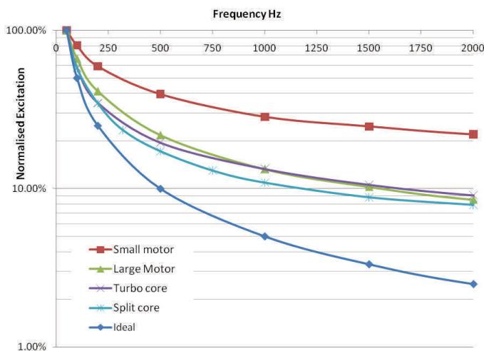
Figure 1. Reduction of excitation current with frequency increase, 50-2000 Hz
