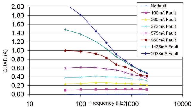
Figure 2. Measured fault current for various faults at different frequencies
