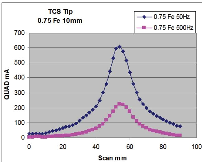
Figure 3. 10 mm long fault on tooth tip
