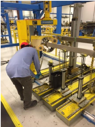
Fig 9 -Operator checking tape tension
