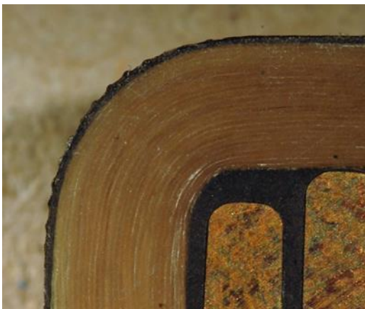
Fig 4 – Cross section of VPI'd bar
