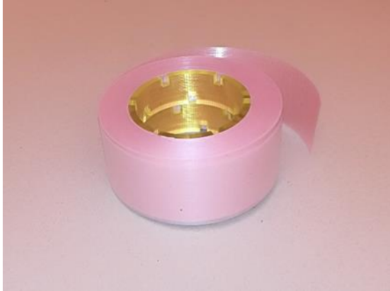
Fig 7 - VPI mica tape roll with catalyst (pink catalyst)
