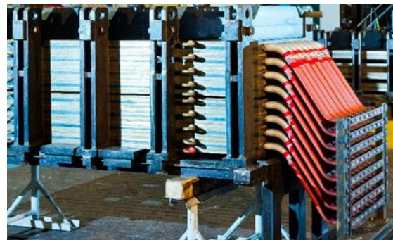
Fig 6 - Typical bar fixture (impregnation mold) for VPI
