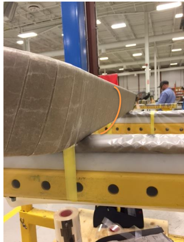
Fig 12 - Taped coil showing the “pillow” effect
