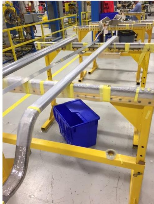
Fig 11- Stator Bar Ready to enter press with sacrifice tape applied
