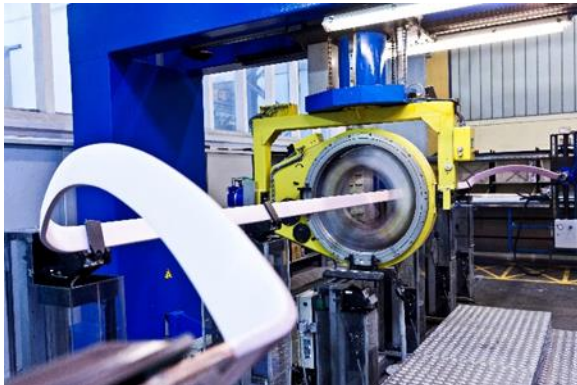
Fig 5 - Taping a VPI bar on a modern 6-Axis taping machine
