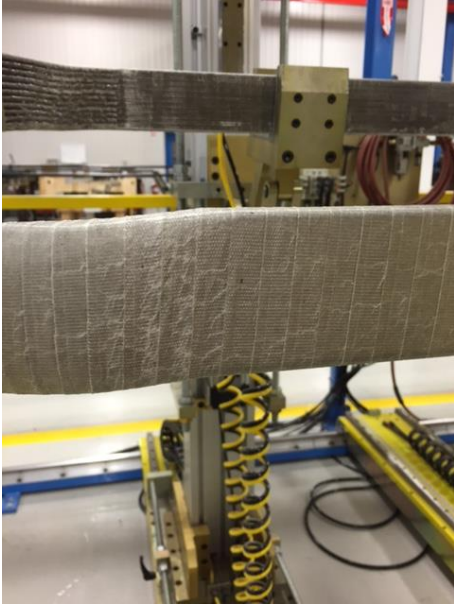
Tape stressed due to offset centerline
