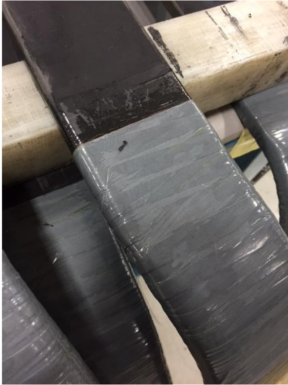
Bar with excellent fit to tooling in press
