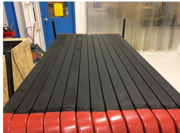
Stator Bar provided for North American customer by Austrian Bar Shop
