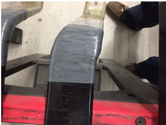
Lack of bend compression and pinch in tape due to mis-match between bar and tooling
