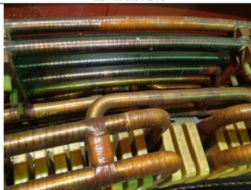
P05: Sections of circuit ring bus discolored
