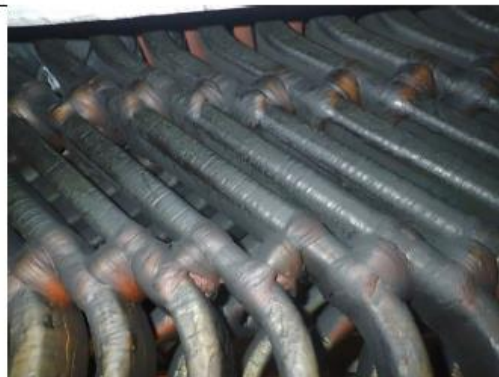
P01: Contamination on bottom end winding
