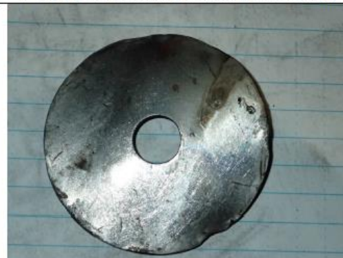
P04: The washer and burn marks possible due to pd between the bars
