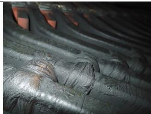
P02: Contamination on bottom end winding
