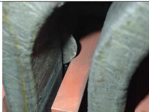
P03: A washer found between front and back bar in slot 245
