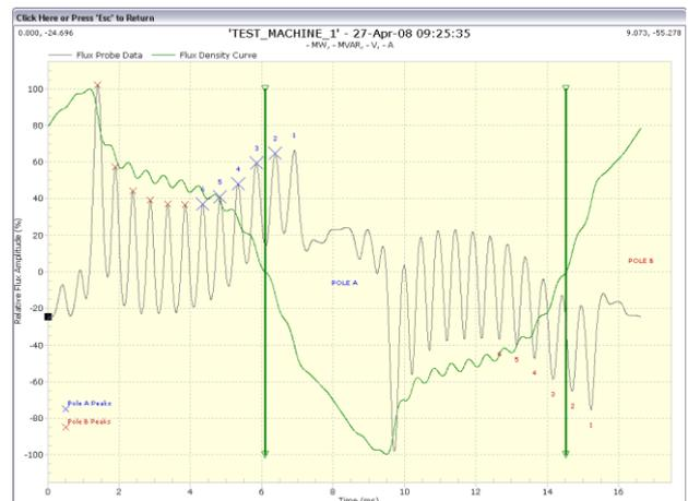
Fig.6 Raw Flux Waveform
