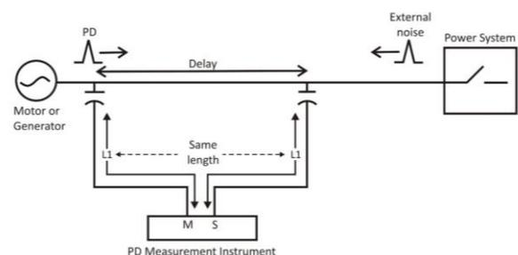
Fig. 3 Time Domain Disturbance Separation by Time of Pulse Arrival [4]
