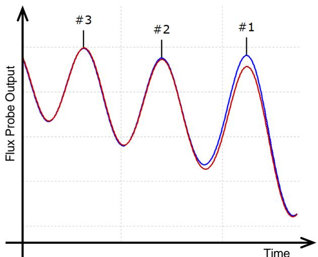
Fig.7 Analysed Flux Data and Peaks show reduced flux at coil number 1
