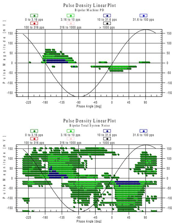
Fig. 4 Phase Resolved PD Patterns of Measurement
