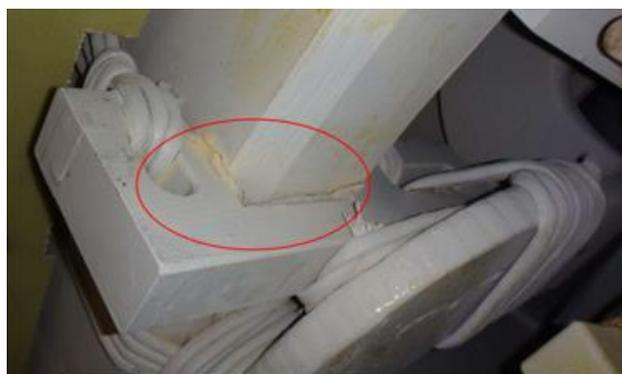
Fig. 15 Dusting and Looseness at One Support Block
