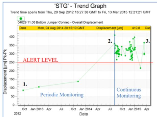
Fig. 14 Trend of On-line Vibration Displacement
