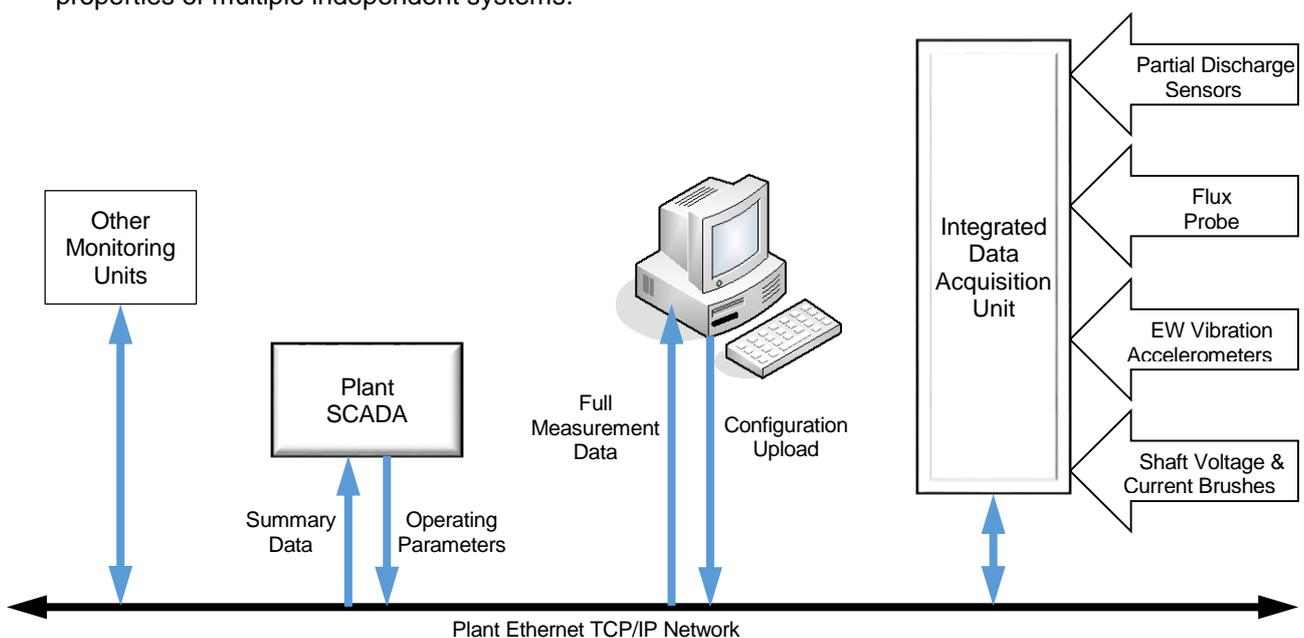
Fig. 10 System Schematic Diagram
