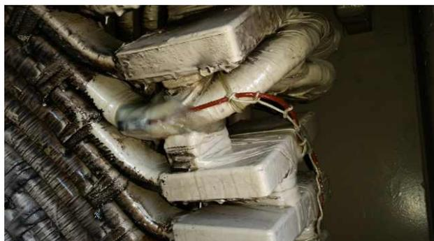
Fig. 9 Accelerometer Installed on Endwinding
