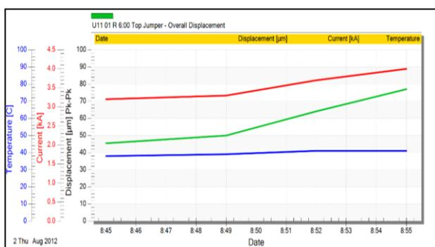
Fig. 11 Endwinding vibration, stator current and winding temperature over time
