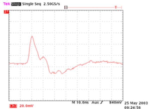
Fig 2 Oscilloscope image of a single PD pulse measured by an 80 pF capacitive PD sensor across a 50 Ω resistor. The vertical scale is 20 mV per division and the horizontal time base is 10 ns per division.
