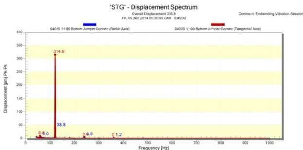
Fig. 13 Displacement Spectrum of Bottom Jumper Near 11 o'clock Position of Stator
