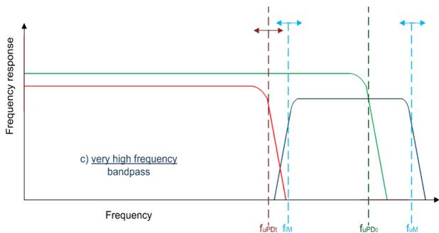
Fig. 1 Idealised Frequency Response of PD Pulse at Source, Noise and Measurement System at VHF Range [4]
