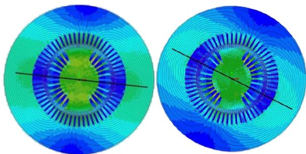
Fig. 8 Magnetic Flux Lines and Shift in Location of Flux Density Zero Crossing at Low Load (Left Diagram) and High Load (Right Diagram) [6]
