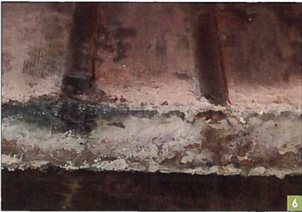
Damaged bar surface due to loose coils in the GVPI stator.
