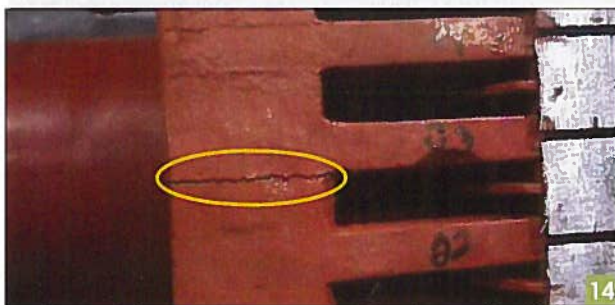
Cracked short-circuit ring. (Photo courtesy of EASA.)
