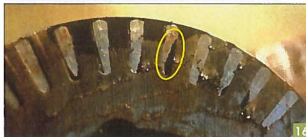
Voids in cast aluminum rotor bars in rotor slots due to poor manufacturing. (Photo courtesy of EASA.)
