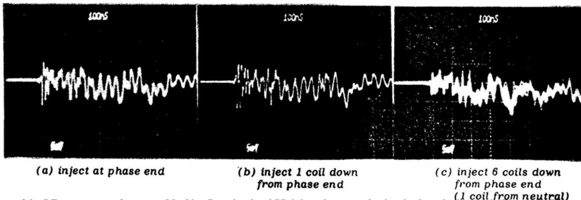
**Figure 7:** Response of the RF current transformer on Machine B to simulated PD injected at several points in the winding (as in Figure 3). The output response is relatively independent of the location of the PD.
