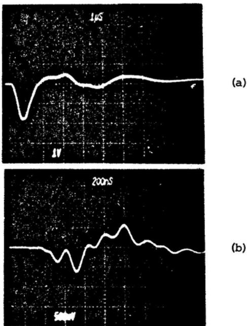
**Figure 8:** RF CT output on Machine B to simulated noise on the (a) slip ring and (b) stator frame (similar to Figures 5 and 6). Note the very high magnitude output compared to Figure 7.
