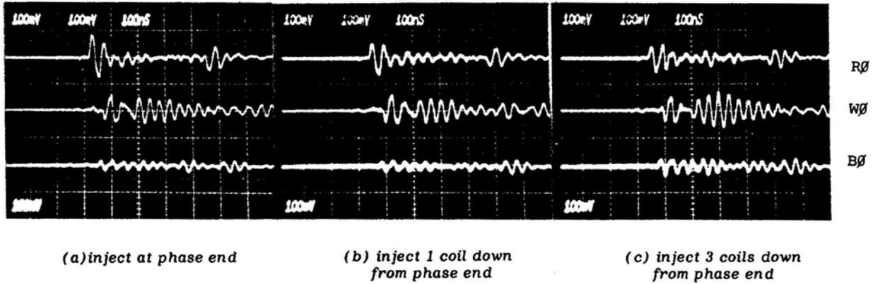
**Figure 3:** Response of capacitive couplers on Red, White and Blue phases of Machine B to simulated PD pulses injected at different points in Red phase. The input voltage is a 100-V, 400-ns wide, 1-ns rise/fall pulse. The important response is the first peak of each waveform; electronic circuitry can ignore the subsequent ringing[4]. As the injection point moves electrically farther away from the terminal, the output response decreases.
