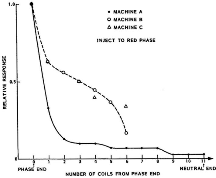
Figure 4: Relative response at the capacitive couplers of three different generators from simulated PD injected at various points in a winding parade!. The phase end response is equal to 1.0. In all cases, the rotor is in the machine.
