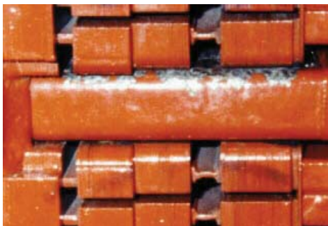
Fig. 4. Major slot PD due to inadequate slot conductive coating system.
