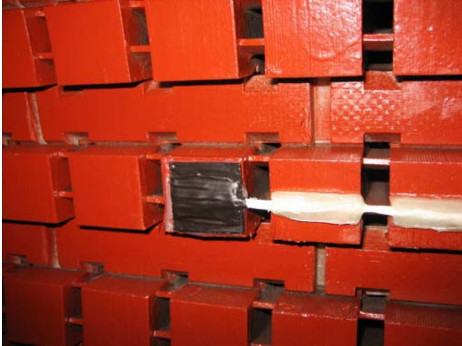
Fig 1: New probe design shown mounted on a stator core tooth
