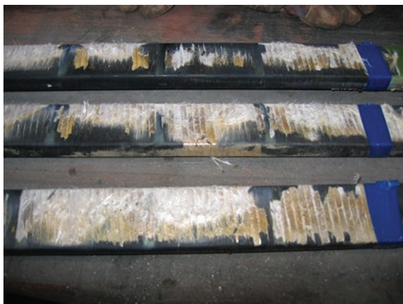
Figure 2. Slot discharge primarily due to poor slot conductive coatings.
