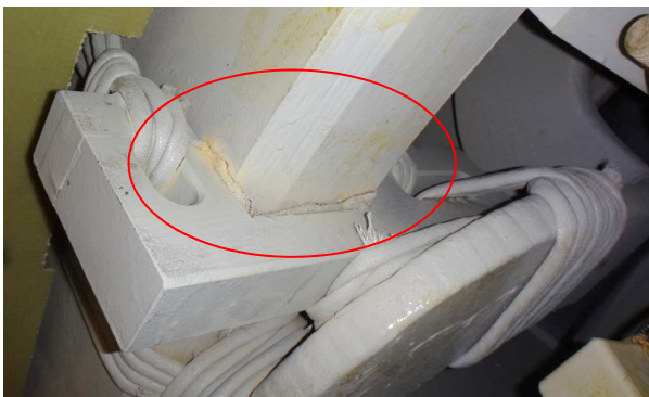
Fig. 8 Visual inspection showing looseness between the support block, circumferential support ring and connection between the winding and circuit ring [9]
