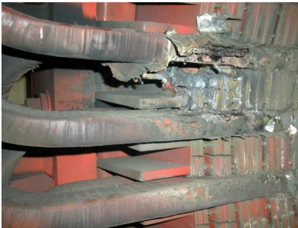
Fig. 3 Collateral damage to the stator winding and core caused by fatigue cracking of the copper conductors due to severe endwinding vibration
