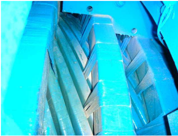
Fig. 2 Photo of insulation abrasion (white powder caused by fretting) caused by relative movement between the coil, support ring, and support brace
