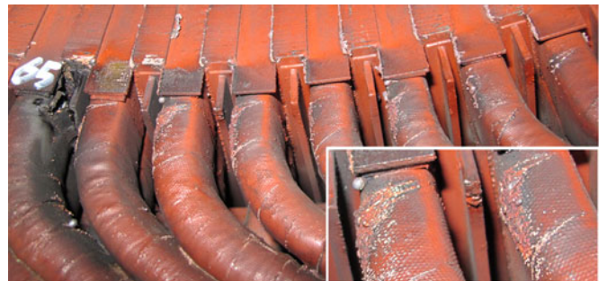
Fig. 5. Turn insulation failure in EW slot exit of 6.6-kV, 1678-kW primary air fan motor (M13) with zoomed in view of melted copper.
