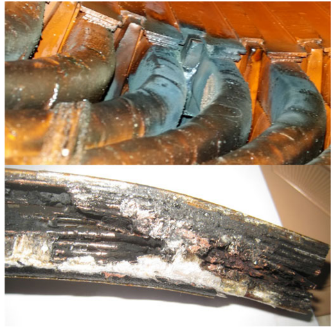
Fig. 3. Turn insulation failure in EW slot exit of 6.6-kV, 205-kW transport blower motor (M9).
