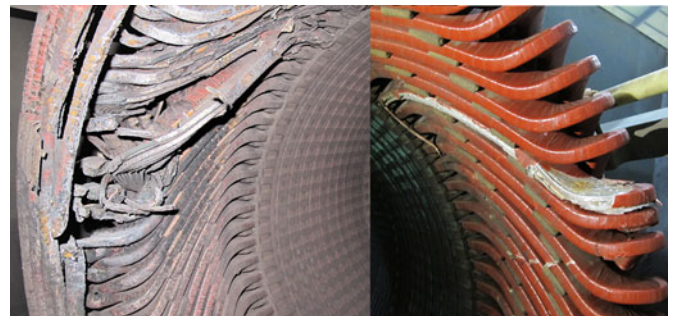
Fig. 10. Phase insulation failure between lead cable and EW of 6.6-kV, 4500-kW boiler feed pump motor (M15).
