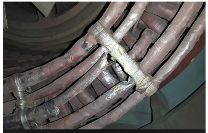
Fig. 9. Phase insulation failure in lead cable of 6.6-kV, 3800-kW boiler feed pump motor (M14).
