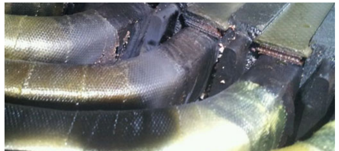
Fig. 4. Turn insulation failure in EW slot exit of 6.6-kV, 310-kW condensate extraction pump motor (M1).
