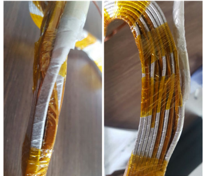
Fig. 12. Example of crossover coil design for 6.6-kV, 75-kW 8 pole motor.
