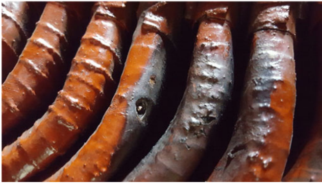
Fig. 6. Turn insulation failure in EW bend of 4-kV, 485-kW primary air fan motor (M12).
