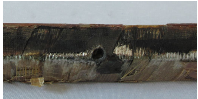
Fig. 1. Ground wall insulation failure in 6.6-kV, 550-kW circulating water pump induction motor.
