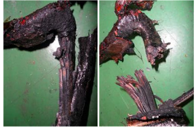
Fig. 11. Turn insulation failure near knuckle of EW of 3.3-kV, 190-kW motor.
