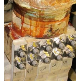
Photo 17. New bolted joint.
