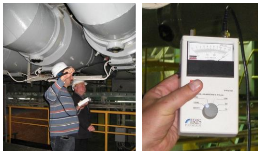
Photos 10a & 10b. PPM 97 measuring a bus EMI source.
