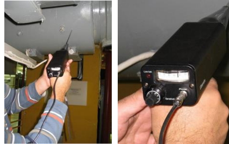
Photos 11a & 11b. Using the Ultraprobe™ assessing the acoustic noise that accompanies EMI
