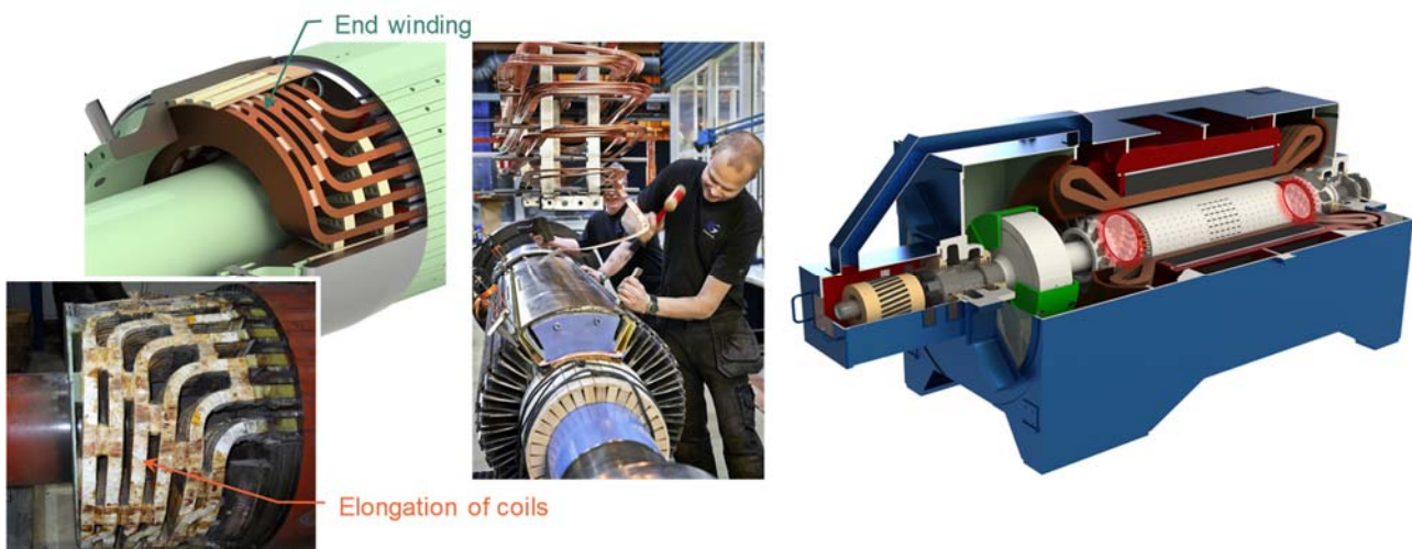
Figure 15 Turn-to-turn short circuits due to elongation of coil end winding is a common failure mode for turbogenerator rotors. But the elongation can also lead to the failure mode earth fault, which is more severe.
