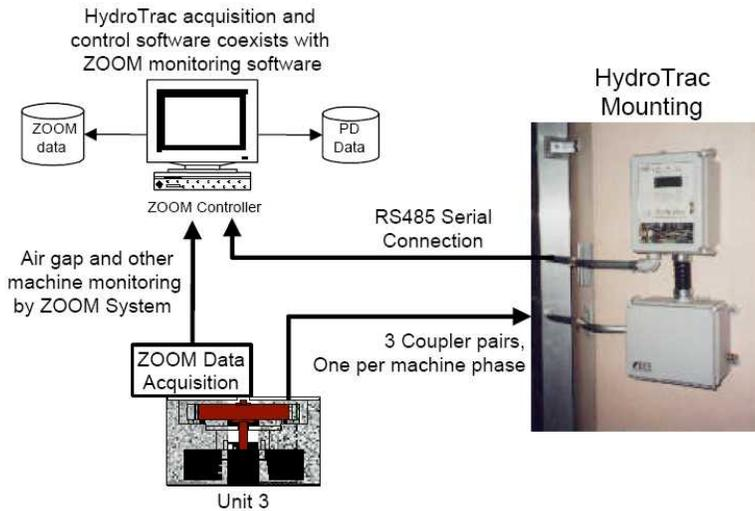
Figure 2. HydroTrac Monitoring System & VibroSystem's ZOOM
