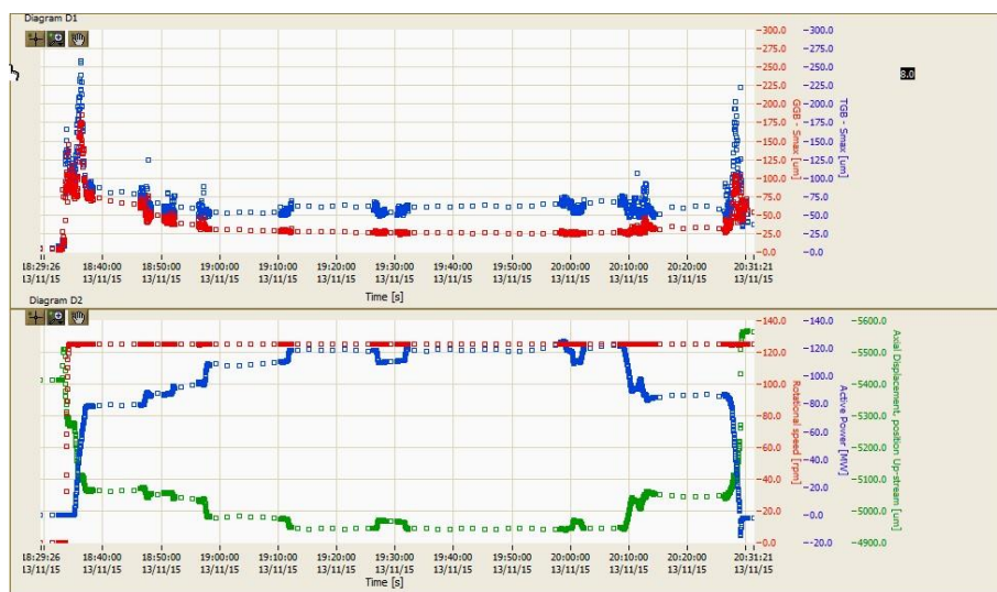
Figure 2 - Upper diagram: Smax @ GGB & TGB; Lower diagram: RPM, Active Power (P) & Axial Displacement.
