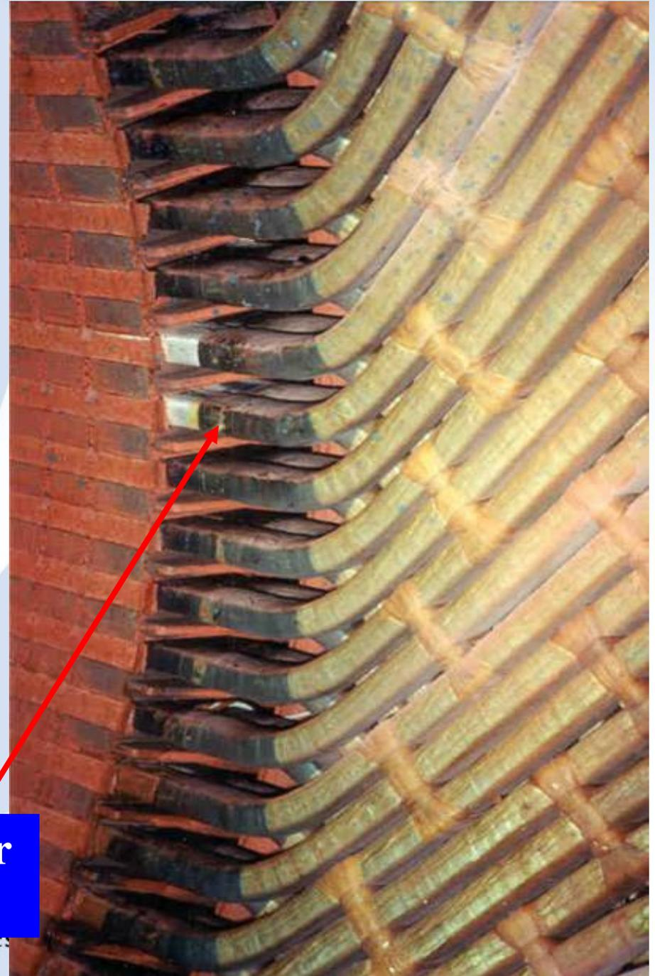
**Surface PD damages due to poor stress grading system**
