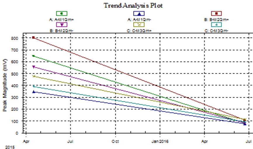
Figure 2 – Trend showing significant drop in PD activity after maintenance
