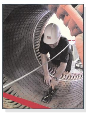
The stator cores of large turbogenerators, hydrogenerators and motors have traditionally been tested using the full flux (ring flux) test. ELCID enables evaluation of the stator core lamination insulation both more safely and faster. This course reviews why stator cores degrade and shows how to perform the ELCID test using the Iris Power Evolution. Examples of calculations and demonstrations are done on a large motor stator. Written and practical testing is done.
