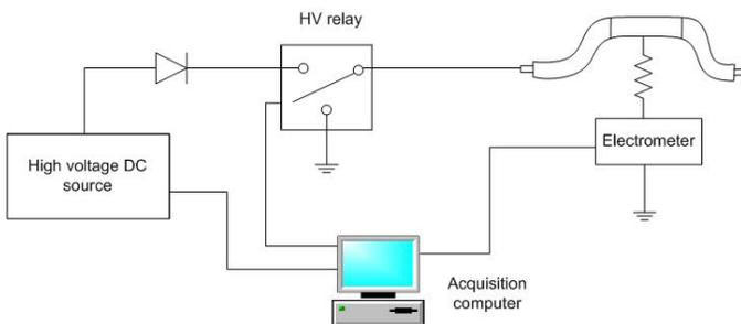
Fig. 1. Laboratory setup for ramp test in UGT mode (adapted from [6]).
