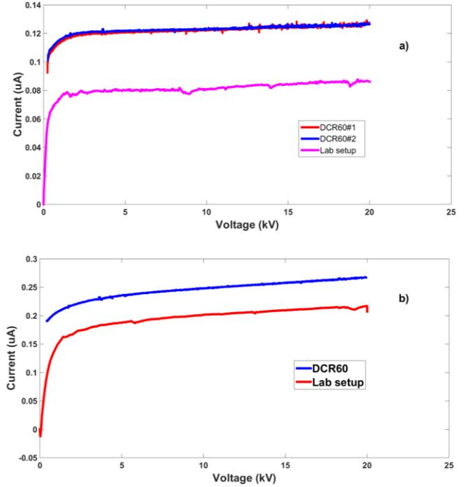
Fig. 2. I-V curves at a rate of 2 kV/min on a a) 2.0 nF b) 4.3 hydro-generator bars obtained from the DCR-60 and from a lab-made equipment.
