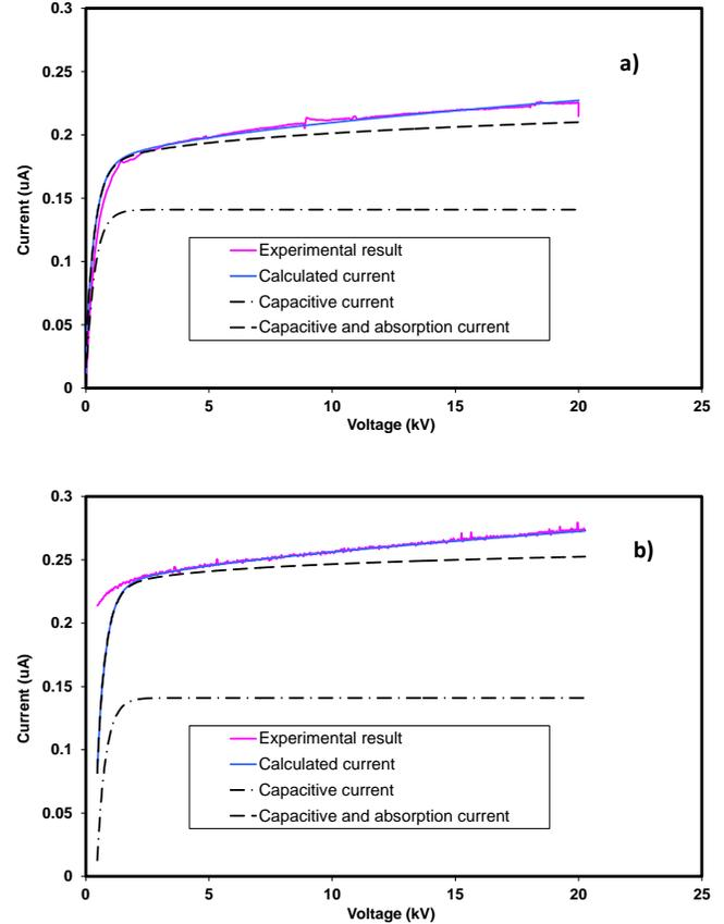
Fig. 5. Modelling (according to eq. 3) of the I-V curve at 2 kV/min on a 4.32 nF bar: a) DCR-60, b) lab setup.
