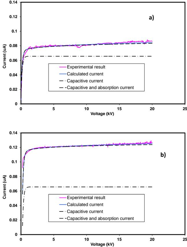
Fig. 4. Modelling (according to eq. 3) of the I-V curve at 2 kV/min on a 2.0 nF bar: a) DCR-60, b) lab setup.
