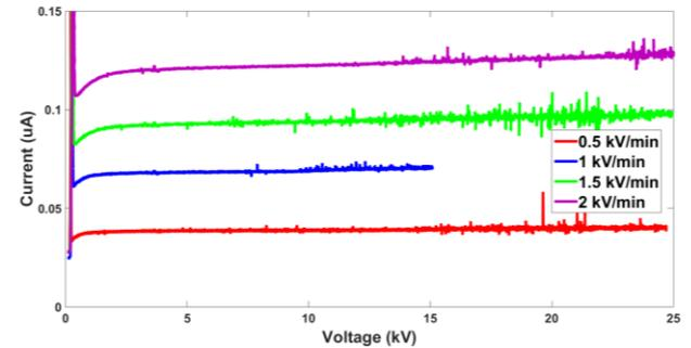
Fig. 3. I-V curves on a 2.0 nF hydro-generator bar measured by the DCR-60 at different voltage rates.
