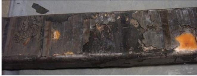
Figure 3a: Observation of the degradation of the semicon coating of Bar L3-1 from Machine 5 (a motor-generator), which had the lowest PDEV and the highest PD magnitudes. This image also shows local burning and PD attack on the bar surface.
