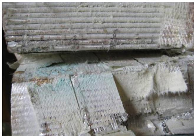
Figure 2: View of turn insulation and conductor stack of coil LC1 from Machine 6. Note that the delamination at the turn resulted in heavy partial discharge attack that further damaged the turn insulation. The green powder is from oxidation of the copper by ozone from the PD.
