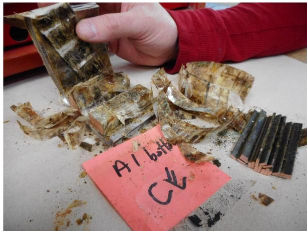
Figure 1: Photographs from the dissection of a segment from Coil A1 from Machine 1. Machine 1 had seen 56 years of base-load operation, but did not experience an in-service failure. Once the axial cut through the groundwall was made, the turns and strands from Coil A1, slot exit (connection end) fell apart. The turn insulation was burned and there was extensive PD attack.
