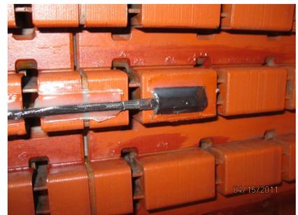
IRIS POWER TFPROBE INSTALLED ON A TURBINE GENERATOR STATOR TOOTH
