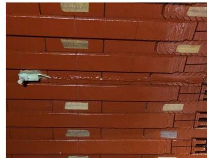
IRIS POWER FFPROBE INSTALLED ON A TURBINE GENERATOR STATOR WEDGE
