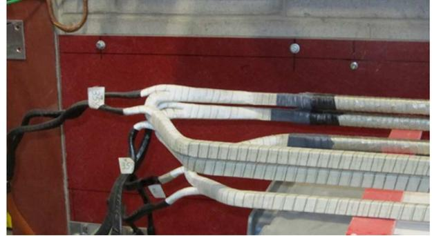
Fig. 4: Photo of three coil model that is connected to a 3 phase voltage supply. The top coil (Phase A) is just a few mm from the middle coil (Phase C)-producing A to C phase PD. B phase is well separated from the other two phases.
