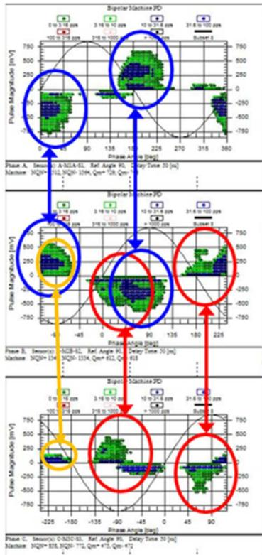
Fig. 3 PRPD examples of interphasal PD occurring between A and B phases (blue circles) and between Phase B and C phases (red circles) on an operating turbine generator, which were confirmed visually on this 80 MVA, 13.2 kV TG. The yellow circle shows signals cross-coupled from A and B phases into C phase. Note the 120-degree phase shift between the start of the AC cycles for each phase, thus the plots are aligned in time.
