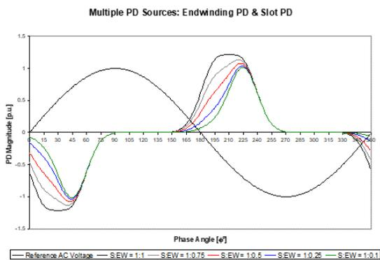
Fig. 2: Simulation of combining void PD with decreasing portions of endwinding PD, causing the PRPD pattern to change its overall shape and mode location. The Gaussian shape is due to voids in the slot alone. The flat top shape in each polarity occurs when void and endwinding PD occurs equally.
