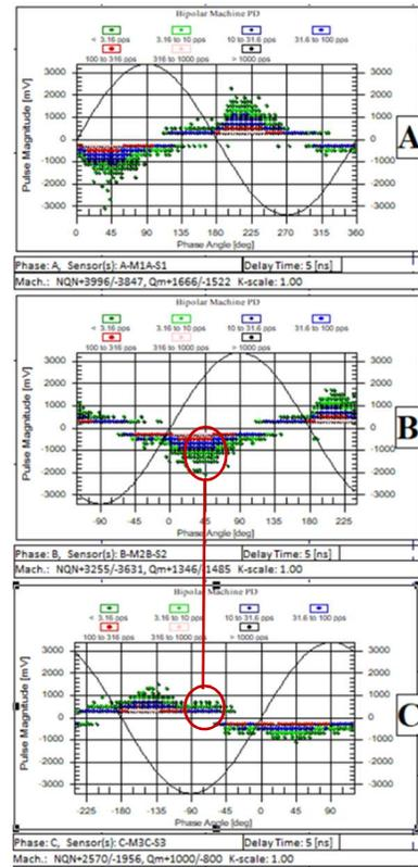
Fig. 5 Cross-coupling into other phases from phase to ground PD only on all three phases. The PD in Phase B is cross-coupled into Phase C – see red circles. There is no interphasal PD due to the wide spacing.
