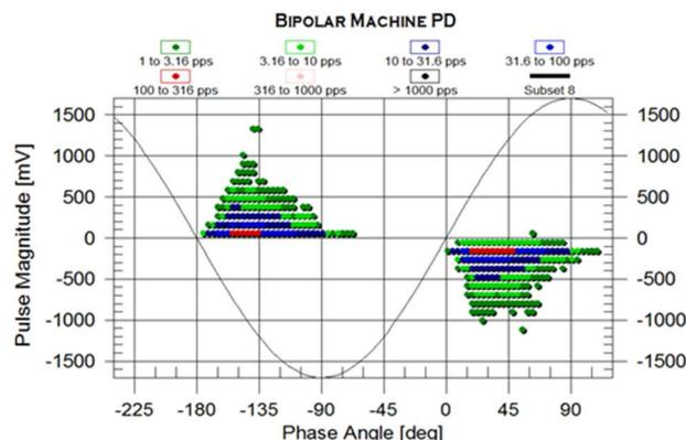
Fig. 1 Classic PRPD pattern caused by a single aging process driven by the phase to ground voltage. The horizontal scale is the phase angle of the 60 Hz AC cycle. The vertical scale is the magnitude of the pulses. The color of the dots represents the PD pulse count per second per magnitude window.
