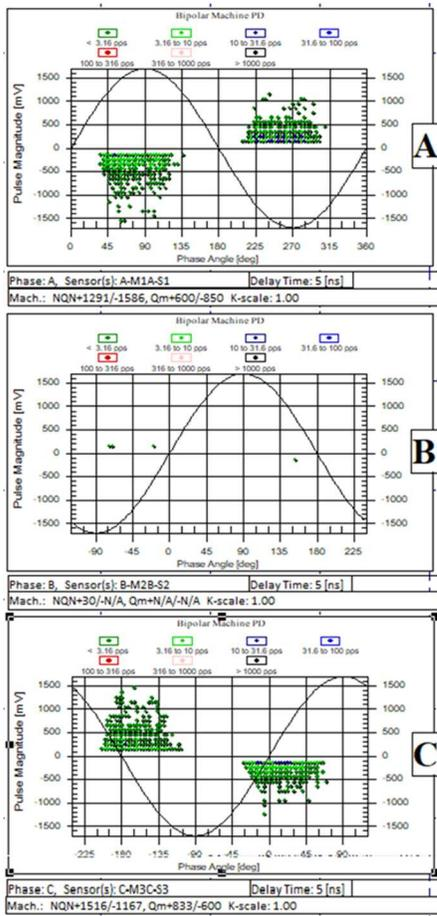
Fig. 6: Pure phase to phase PD between A and C phases. All three phases are energized to 6.9 kV phase to phase.
