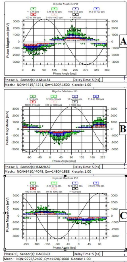
Fig. 7 Void PD in the slot and A to C interphasal PD occurring at the same time.
