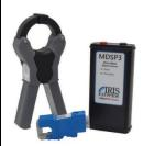
Portable instrument to detect motor rotor cage winding faults and air gap eccentricity
