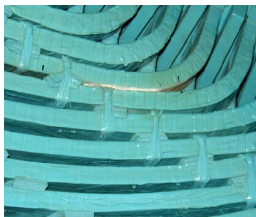
Figure 1: The white powder is the result of high PD activity in the endwinding of a large air-cooled generator where the stator bars in different phases were installed too close to one another.
