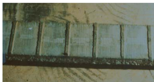
Figure 2: Coil removed for a stator where the coils became loose during operation. The result was that rubbing against the stator core abraded the insulation on the coil sides, and PD ensued.
