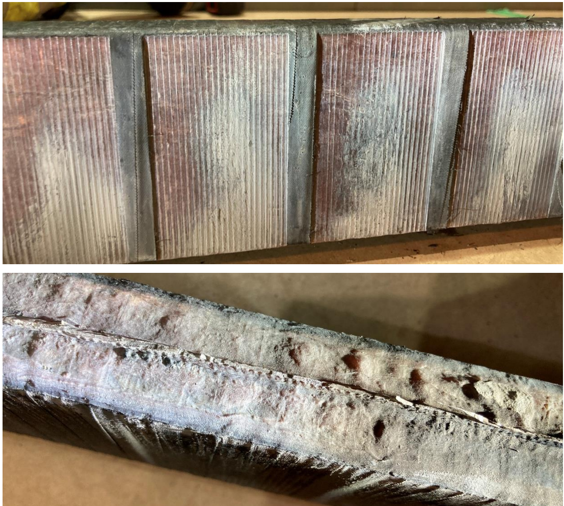
Picture 5. Failed bar of Case 2. Bottom of the top bar was punctured (lower picture). The line in the middle of the bottom is caused by the structure of the filler strip between top and bottom bar and is not a feature of the insulation system. No clear signs of sparking (slot discharges or vibration sparking), the erosion appears to be mechanical.
