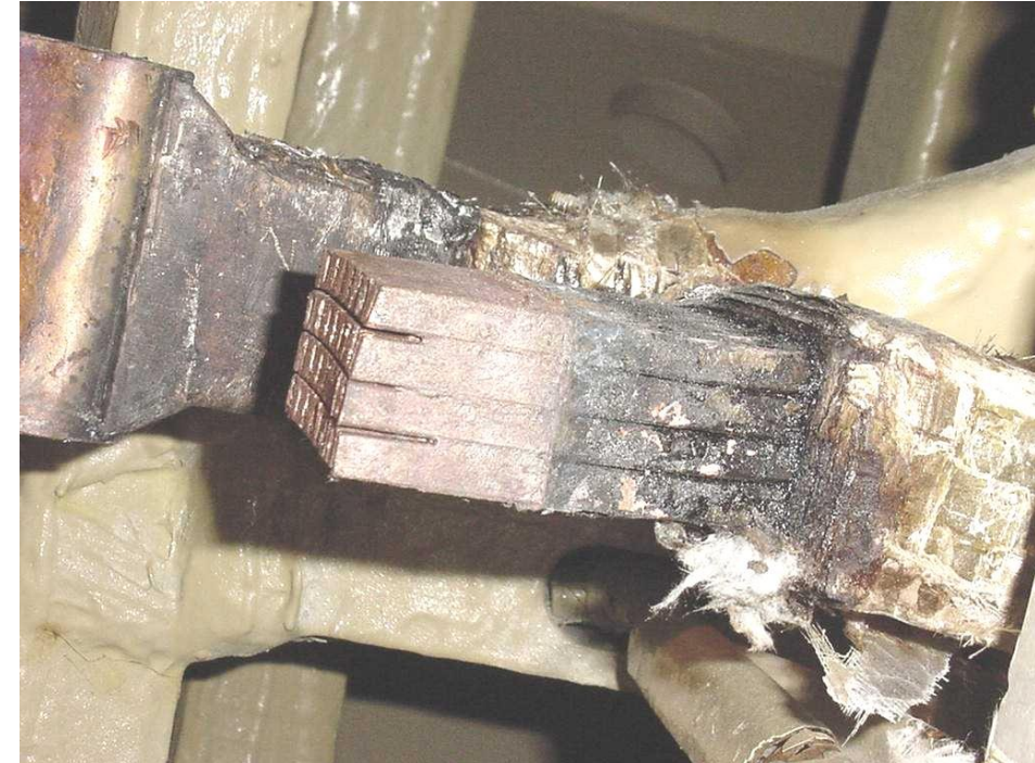
Coil strand package with clip removed
