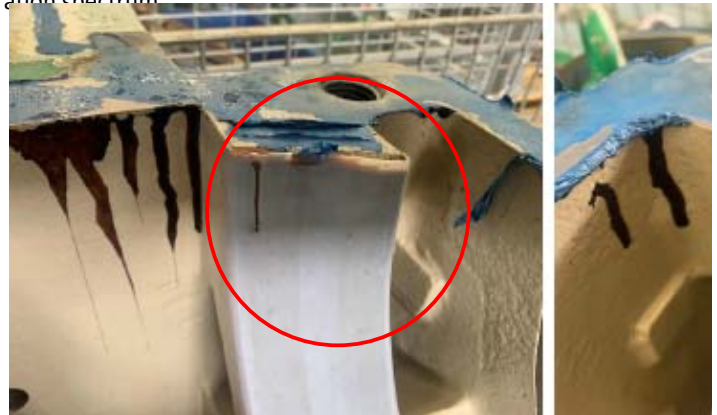
Oil staining on the bearing seal on both sides of the shaft was evident
