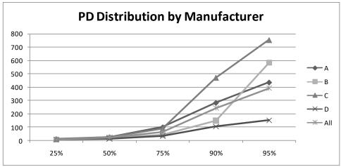
Figure 1. PD Magnitudes based on Manufacturer for 3-5kV Machines
