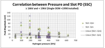
Figure 4. SSC Slot -- PD correlation with Pressure for Manufacturer D for windings installed before 1990 (≥16 kV-19 kV)
