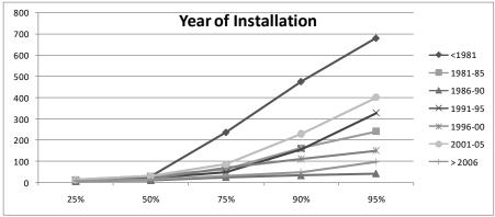
Figure 2. PD Magnitudes based on Year of Installation for 3-5 kV Machines
