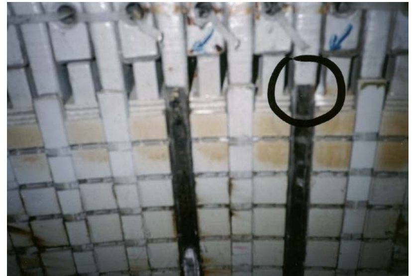
PD on semi-conducting and gradient coating connection (coating deterioration)
