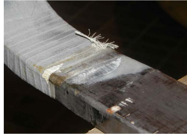
PD on semi-conducting and gradient coating connection (coating deterioration)
