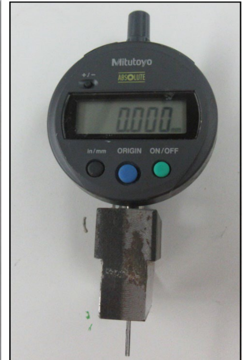
Mitutoyo ID-S112MX electronic Depth Gauge
