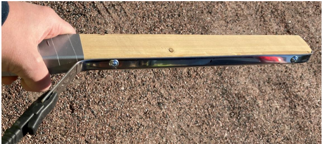
Picture 6. Wooden tool made to bring the stainless steel electrode with the electrolyte pad on the bottom of the slot. This is connected to the minus pole of the DC source. The stainless steel electrode is not corroded in the process.
