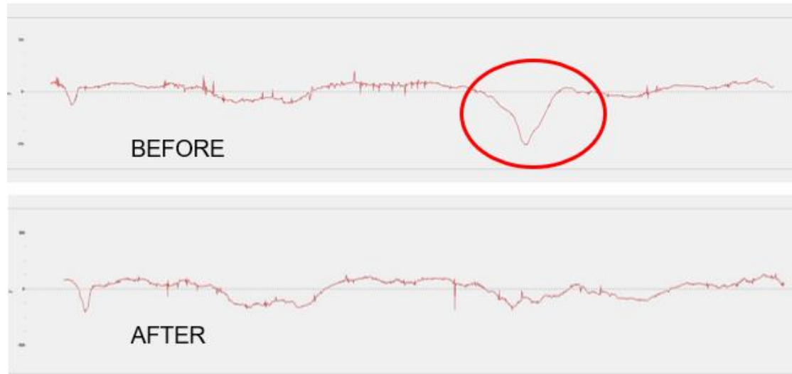
Picture 11. ELCID measurement confirms the core fault indication I_{\text{quad}} = 130 \text{ mA} has disappeared.
