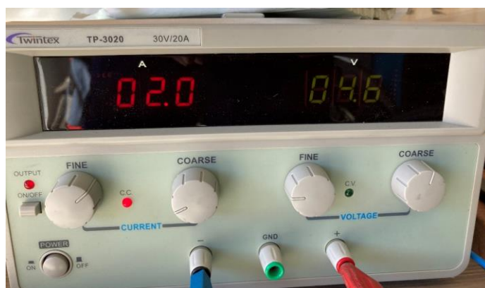
Picture 9. A standard inexpensive laboratory DC source was used for the electrolysis.
