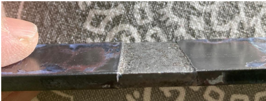
Picture 5. Test etching on a piece of structural steel. The area 30 mm x 18 mm in the middle was etched appr. 4 h with low 2 A DC current, which removed some 0,2 – 0,3 mm of the steel surface.
