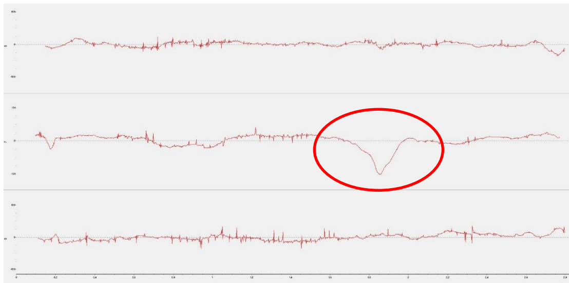
Picture 4. ELCID I_{quad} curves of the damaged stator core slot (in the middle) and two neighbor slots. Deviation I_{quad} = 130 mA indicates a possible local hot spot 5 – 10 °C in normal operation.
