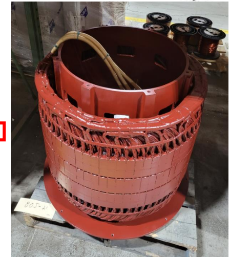
Exciter rotor supplies AC output to the diode wheel
