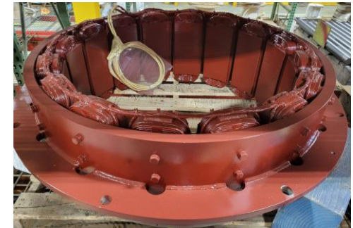
The exciter stator induces current in the exciter rotor
