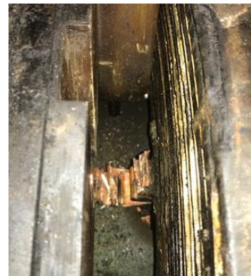
Cracked J-Strap above & Severed & Tested Below
