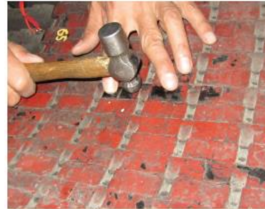
Figure 6. Wedge tap test for tightness
