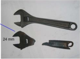
• Two pieces of an adjustable wrench found between top and bottom coil in end winding area. Also a pen was found in the area.
