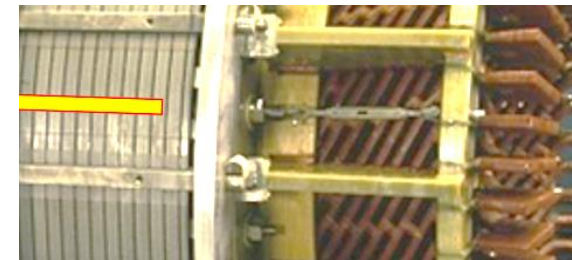
Missing nut (10-12 O'clocks seen from Turbine)
