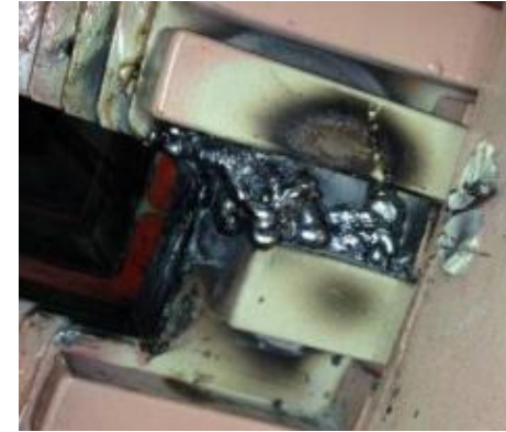
Photo of first unit failed & typical arc location above. TGUG 2017. Progression of arc damage on host unit below.
