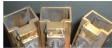
Figure 20. Carbon dust in brush holder
