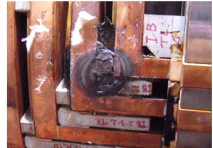
Two cases of extensive damage from ground faults.
