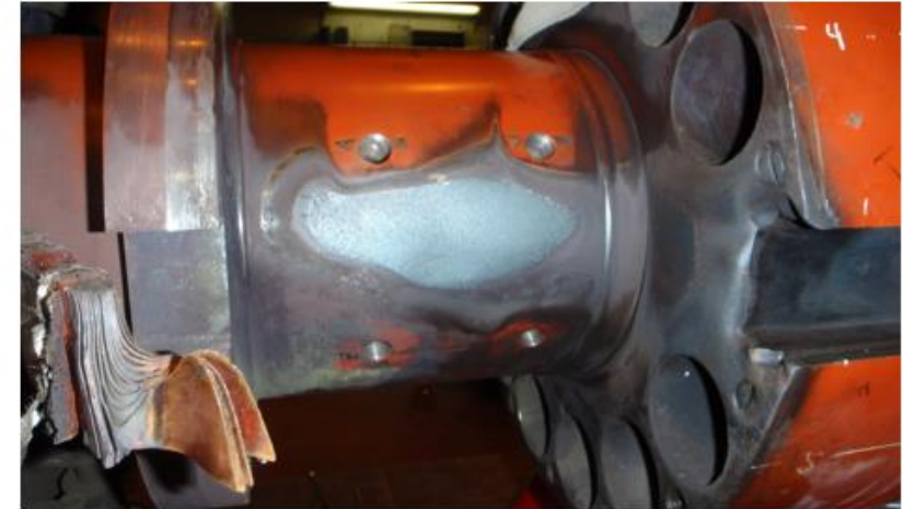
Two cases of extensive damage from ground faults.
