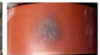
Images from 30020246 showing typical location of generator CTs, type of construction and common heat damage failure mode.
