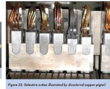
Figure 22. Selective action illustrated by discolored copper pigtail
