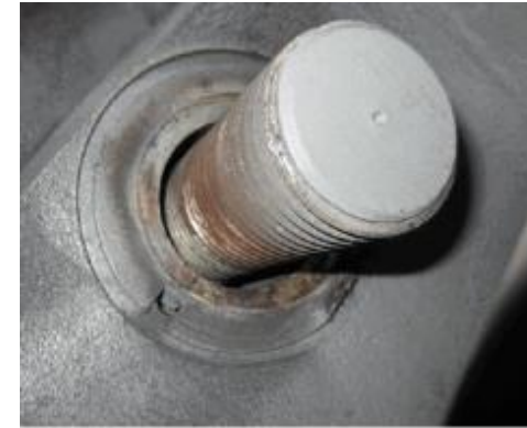
Missing nut (10-12 O'clocks seen from Turbine)
