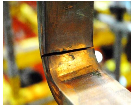
Cracked J-Strap above & Severed & Tested Below
