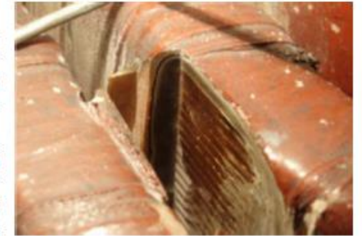
Figure 1. Generator stator coil shown with abraded copper strands and ground insulation due to repeated-load cycling. The support block that abraded into the coil is not shown. [1]
