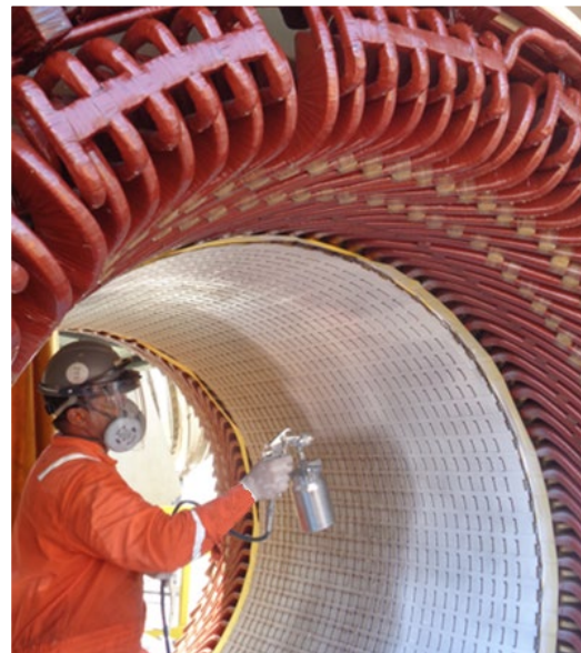
Complete cleaning and painting stator/rotor
