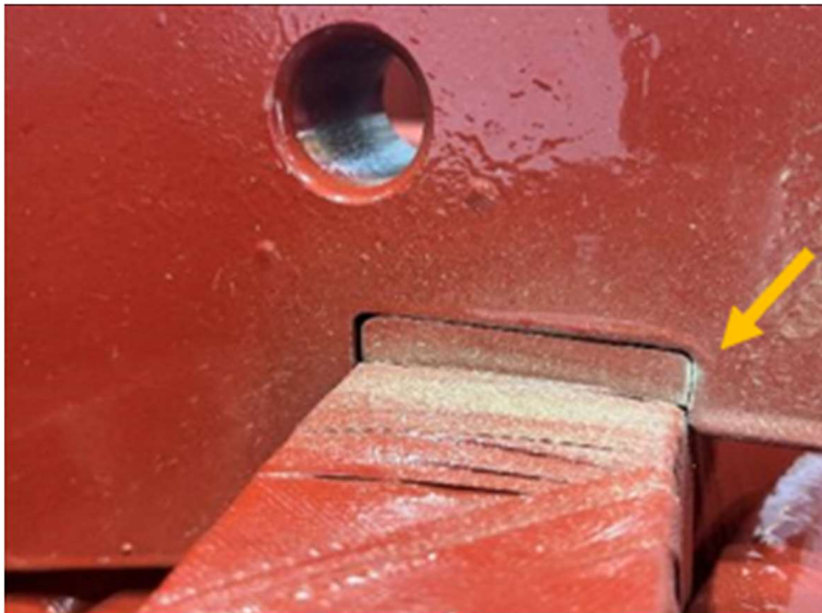
Figure 3 –DE Endwinding – Indication of Dusting
